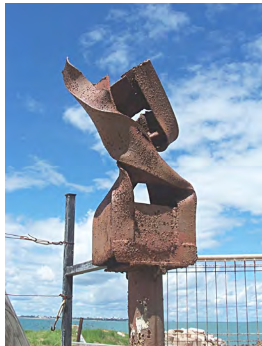
The base of a steel electricity pole bent by Tracy
