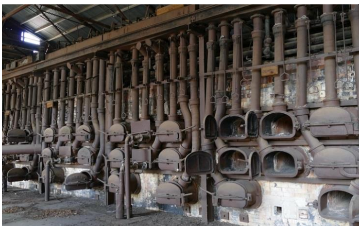
Left: The horizontal retorts and ascension pipes in the retort house at Fakenham gasworks, the only complete example of a town gasworks in England. Image: Historic England Archive Below: Retort House, Bendigo Gas Works. Image: Bendigo Branch
