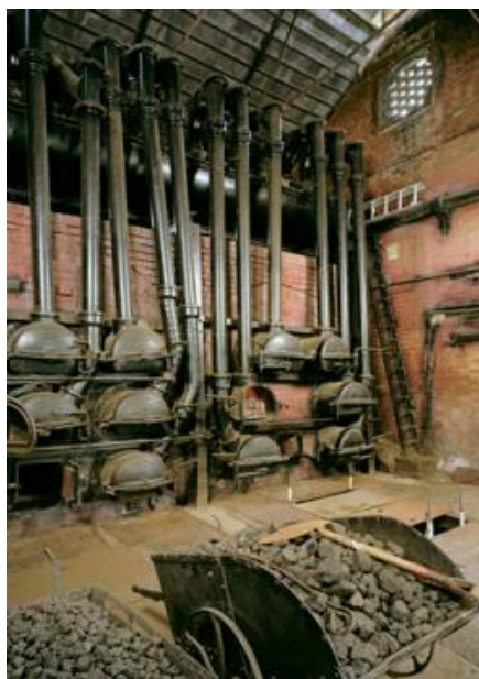
Left: The horizontal retorts and ascension pipes in the retort house at Fakenham gasworks, the only complete example of a town gasworks in England. Image: Historic England Archive Below: Retort House, Bendigo Gas Works. Image: Bendigo Branch
