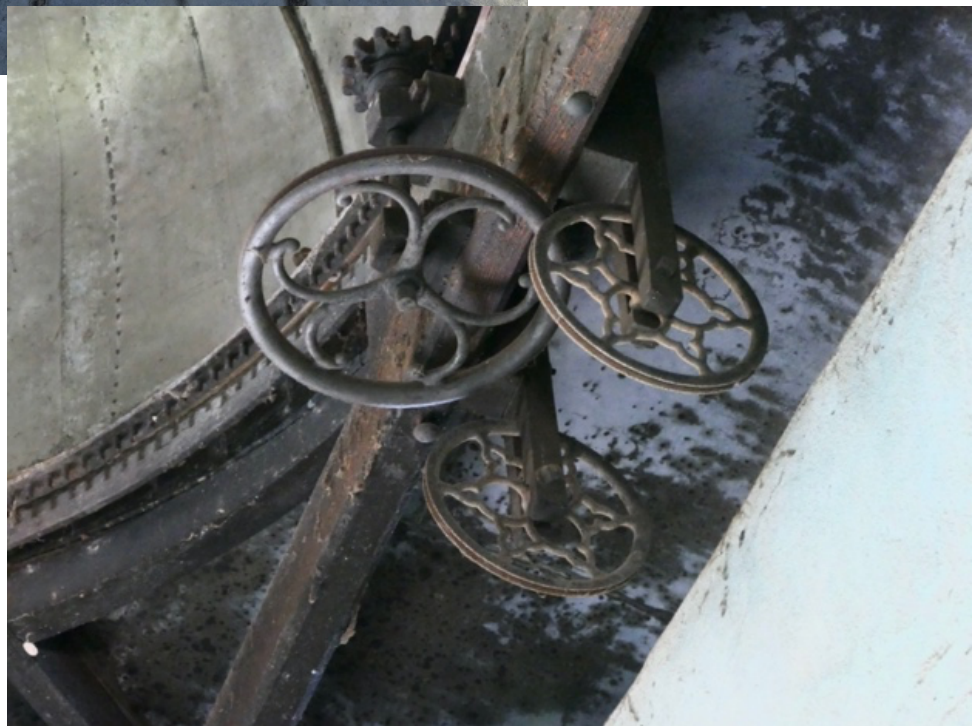
Inside the telescope dome, looking up. Detail of winding mechanism to open dome
