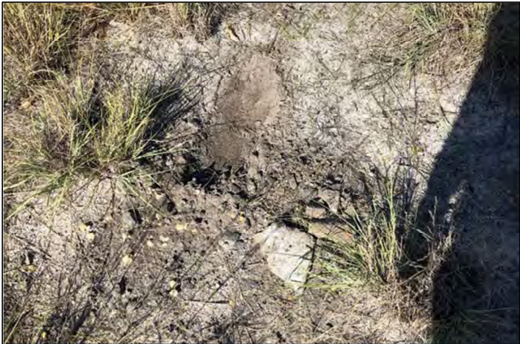
Plate 21: ACM observed in the fill material in Lot 561.
