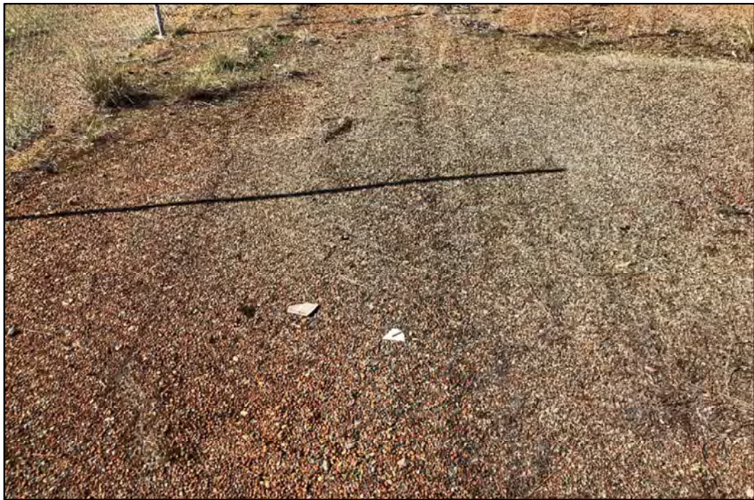
Plate 4: ACM fragments on the surface soil of one of the access tracks to the south of the Roundhouse
