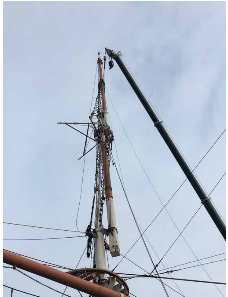
Lifting away the two mast sections of the mainmast
